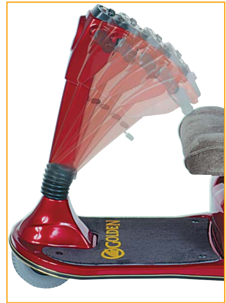
Patented infinite adjustable tiller
